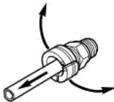
Fig. 129: OIL COOLER LINE QUICK CONNECT FITTING - DISASSEMBLY
