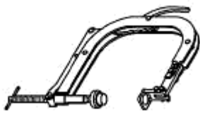
Fig. 73: Valve Spring Compressor C-3422-D Courtesy of CHRYSLER LLC
