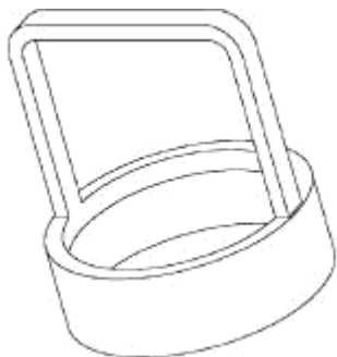
Fig. 275: Compressor, Spring - 8250 Courtesy of CHRYSLER LLC
