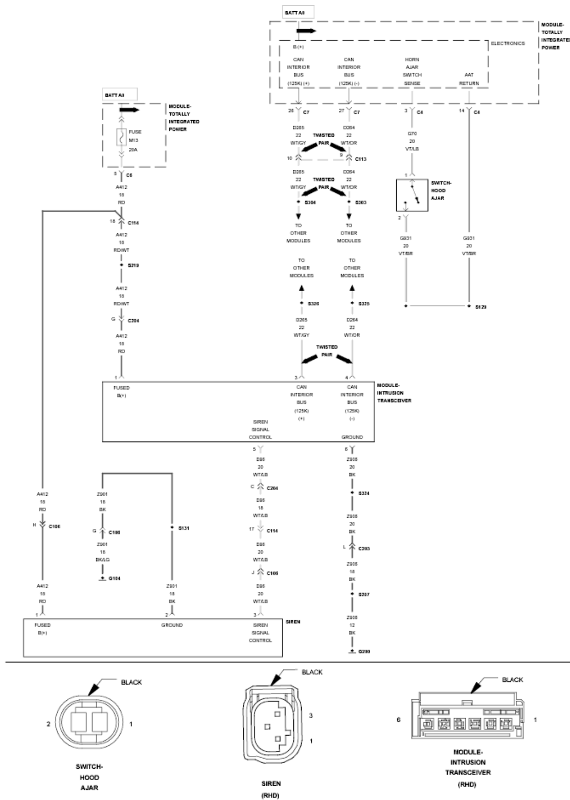
Fig. 56: ITM CAN Interior BUS, Fused B(+) & Ground Circuit Schematic Courtesy of CHRYSLER LLC
